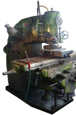
Vertical movable working bench milling machine WM-X5040A 400*1700mm Accuracy: 0.05mm
