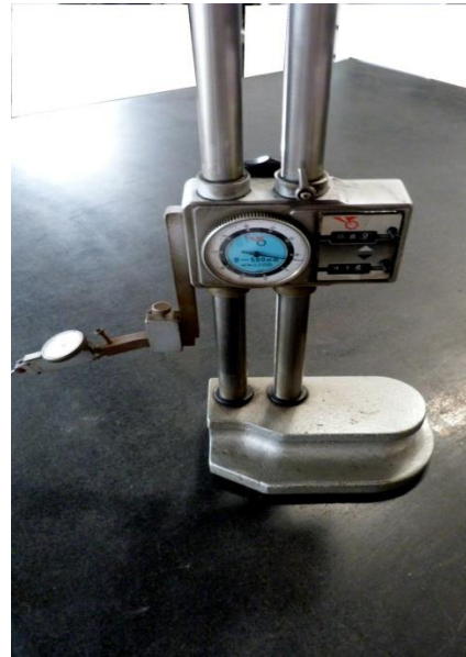
Height gauge:500mm Accuracy: 0.01mm
